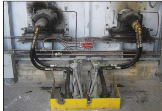
1 kg of Chesterton 615 HTG is used to grease the bearing per year...or <6% of bearing cost.
