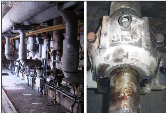
Continuous casting of stainless steel is harsh on roller table bearings.
